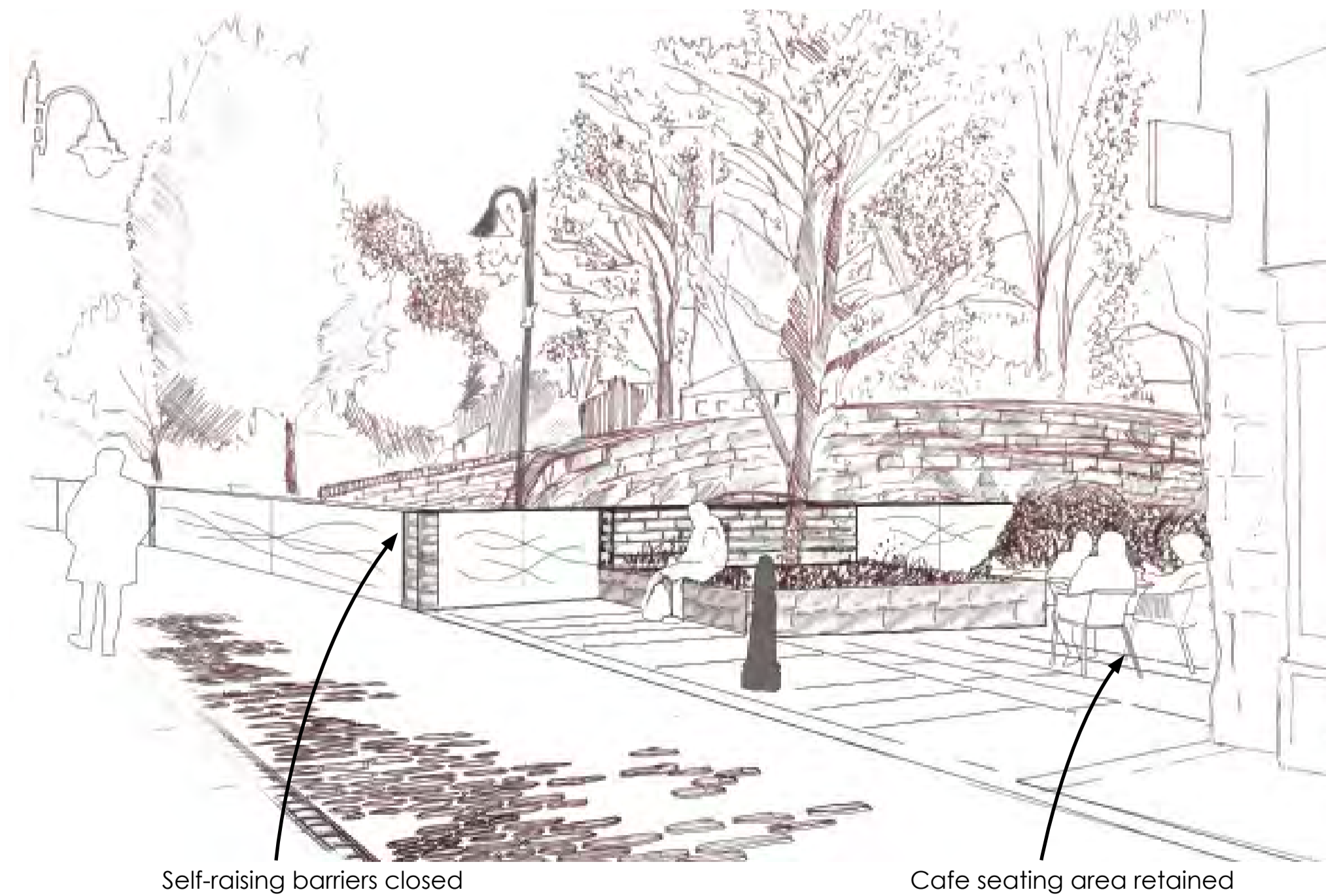
Option 1 - Bridge Gate: Self-raising walls and fixed walls. Raising walls to be embedded in existing foot ways and entrances, with fixed stone walls to follow alignment of existing planting areas.
